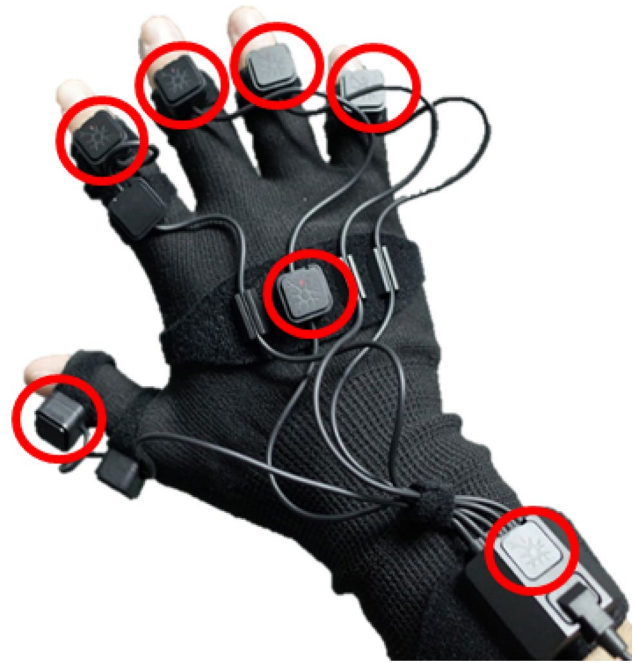
Fig. 3 Glove sensor used in the data collecting process. Five fingertip sensors, a palm sensor, and a forearm sensor are used to describe patterns. IMU sensors are used in this glove
